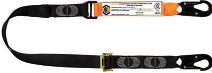
The PIP Adjustable Lanyard with shock absorber are used in various fall arrest situations and is designed protect a worker up to 150Kg. The Webbing is UV rated to meet AS/NZS 1891.5:2020 standards.
