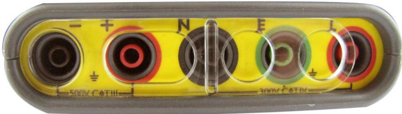
Fig.1 Interlock in position for Continuity and Insulation testing
