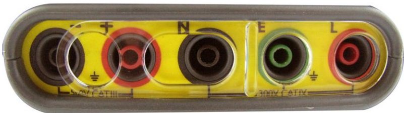
Fig.2 Interlock in position for RCD & Loop testing
